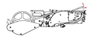
2.Open protect clasp,put the tape to get through tape guide assy.
