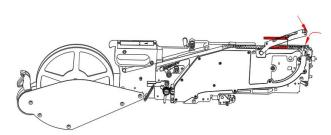
4.Pull the membrane and press the tape guide assy, lock the protect clasp.
